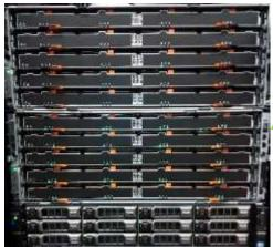
60 HDD auxiliary chassis
